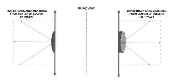
b. The setback for bridge *structures* and culverts with widths or diameters greater than 10 feet, shall be measured from the outside perimeter of the opening, as shown by the red arrows in the diagram below.
